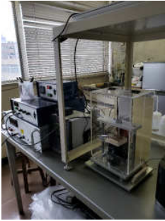
Brand-new installed. For measurements of both electric polarization and piezo-strain vs. external applied electric field.
