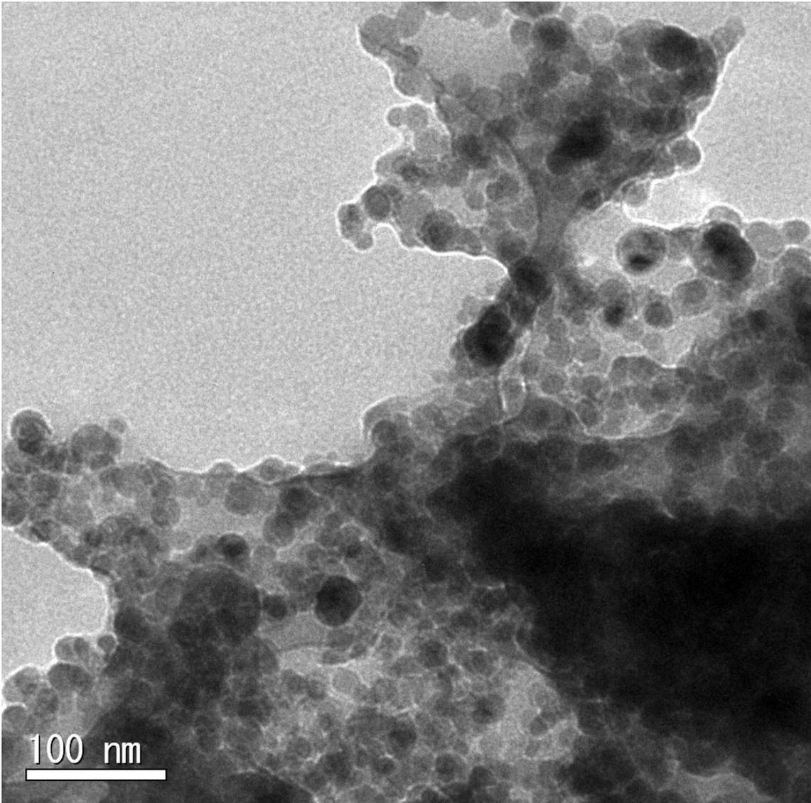
TEM bright field image of nanoparticles of an alloy. Application to Na cooling for Fast Breeding Reactors.
