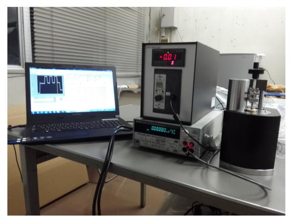
d33 meter for room temperature hot stage up tp 400°C, d31 and d15 attachments, later maybe
