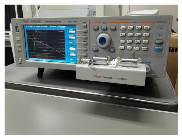
LCR impedance analyzer room temp. 100Hz·1MHz enough for detecting resonance and anti-resonance a new one is coming, its max 4MHz, hot-stage installed, T=room temp.·800degreesCmax, data saved to usb
