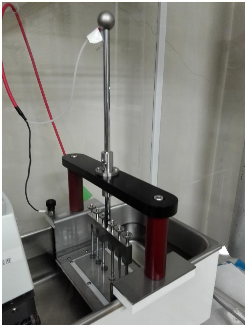
polarization treatment apparatus
